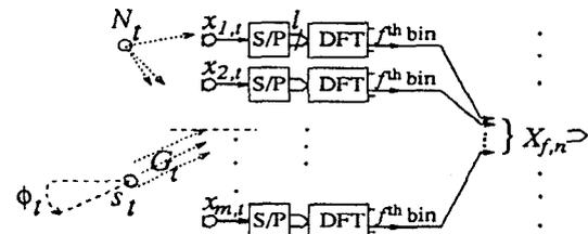
Figure 1. Serial to parallel and transform to the frequency domain of the observation signals.
