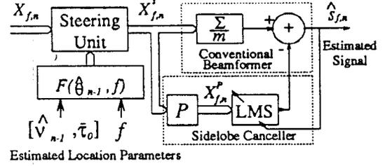
Figure 2. Beamforming unit of the algorithm in the frequency domain with the GSC structure at the frequency  $f$ .
