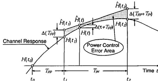
Figure 3: Piecewise-linear power control with channel response prediction.
