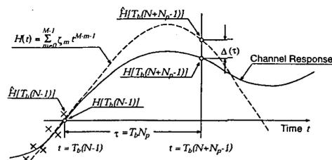
Figure 2: Pairwise observations on  $(T_b n, \hat{H}(T_b n))$  constitute a scatter diagram. The relationship between  $T_b n$  and  $\hat{H}(T_b n)$  is approximated by a polynomial function.
