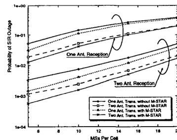
Figure 4: Effects of modifications to STAR on the probability of SIR outage vs. cell loading.
