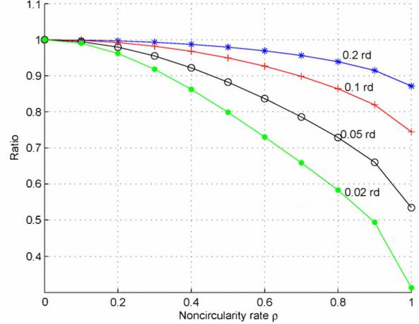
Figure 5. Ratio =  $(\text{CRB}^{\text{noncir/cor}}) / (\text{CRB}^{\text{cir/cor}})$  as a function of the noncircularity rate  $\rho$  for different values of DOA separation ( $\Delta\theta$ ), for  $\phi_1 = \pi/2$ ,  $\phi_2 = \pi/3$ ,  $N = 100$  and  $\text{SNR} = 0\text{dB}$ .
