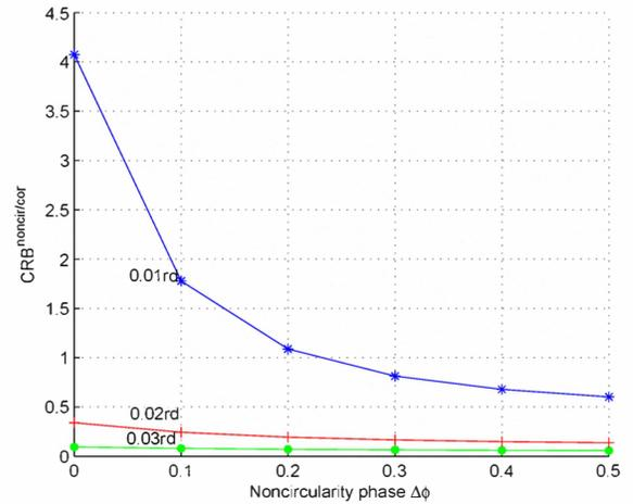
Figure 6.  $\text{CRB}^{\text{noncir/cor}}$  as a function of the noncircularity phase  $\Delta\phi$  for different values of DOA separation ( $\Delta\theta$ ), for  $\rho = 1$ ,  $N = 100$  and  $\text{SNR} = 0\text{dB}$ .
