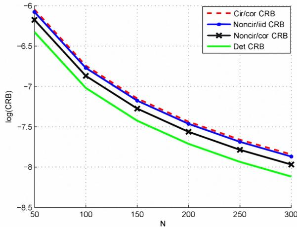
Figure 2. CRBs versus the number of snapshots  $N$  in logarithmic scale for two equipowered sources.
