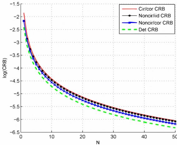
Figure 1. An example of the CRBs versus the number of snapshots  $N$  in logarithmic scale for two equipowered sources.
