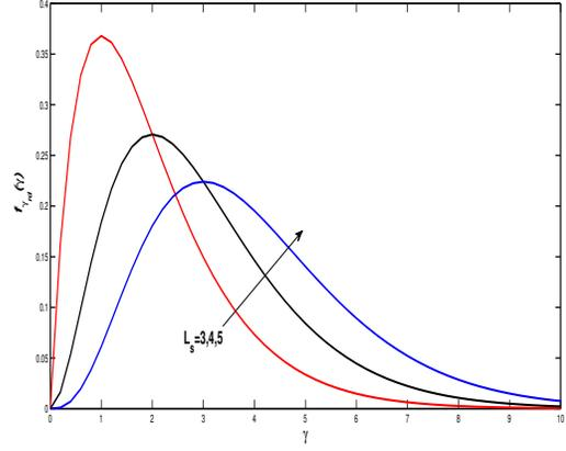
Fig. 2: PDF of the received SNR at SD,  $f_{\gamma_{rd}}(\gamma)$ .
