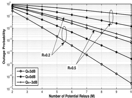
Fig. 4: Outage Probability vs. number of potential relays for  $Q = -3, 0, 3$ dB for both  $R_{min} = 0.2, 0.5$  bits/s/Hz.
