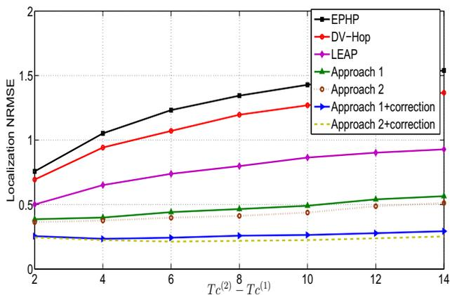
Fig. 6. Localization NRMSE vs. deviation between transmission capabilities.
