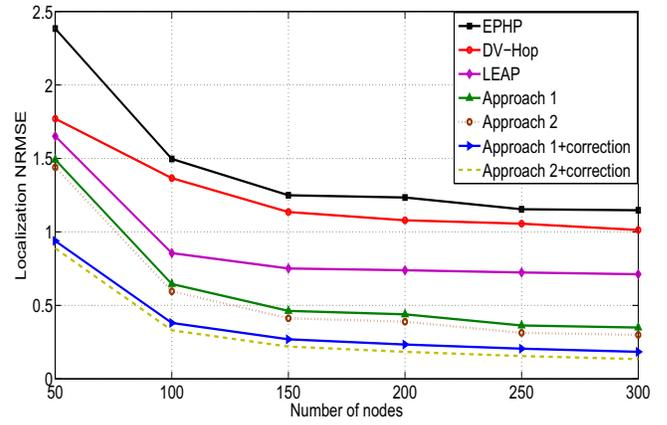
Fig. 4. Localization NRMSE vs. number of nodes.
