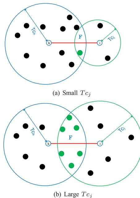
Fig. 2. Effect of intermediate node transmission capability.
