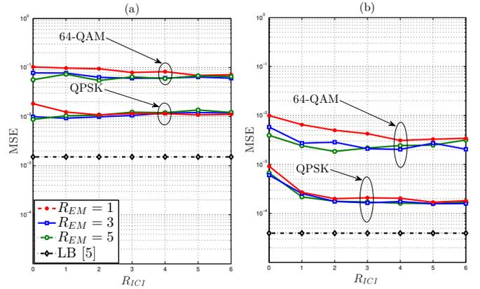
Fig. 1. MSE of ML EM vs its number of iterations with  $N_c = 3$  and  $N_p = 8$  at: (a)  $\text{SNR} = 10$  dB, and (b)  $\text{SNR} = 30$  dB.
