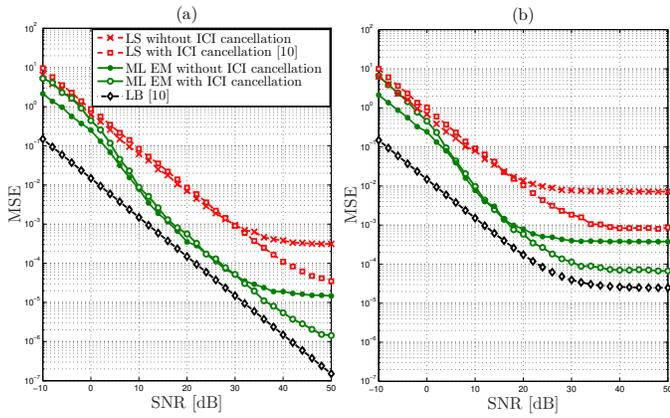
Fig. 2. MSE of ML EM and LS vs. the  $SNR$  with  $N_c = 3$  and  $N_p = 8$  at: (a)  $F_D T = 0.02$ , and (b)  $F_D T = 0.1$ .
