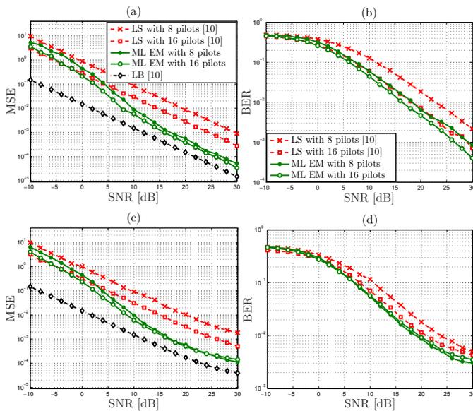
Fig. 3. MSE and BER of ML EM and LS vs. the  $SNR$  with  $N_c = 3$  in terms of: (a) MSE at  $F_D T = 0.02$ , (b) BER at  $F_D T = 0.02$ , (c) MSE at  $F_D T = 0.1$ , and (d) BER at  $F_D T = 0.1$ .
