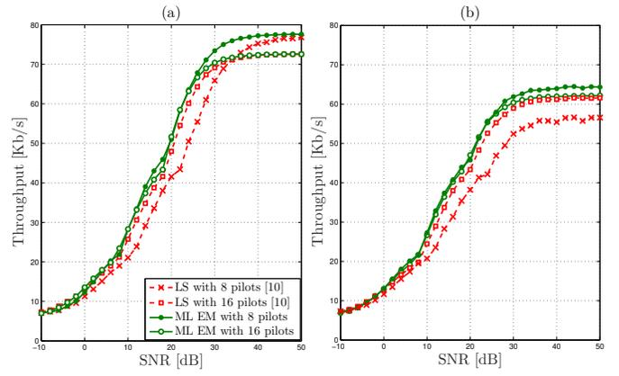
Fig. 4. Link-level throughput vs. the  $SNR$  for ML EM and LS at: (a)  $F_D T = 0.02$ , and (b)  $F_D T = 0.1$ .
