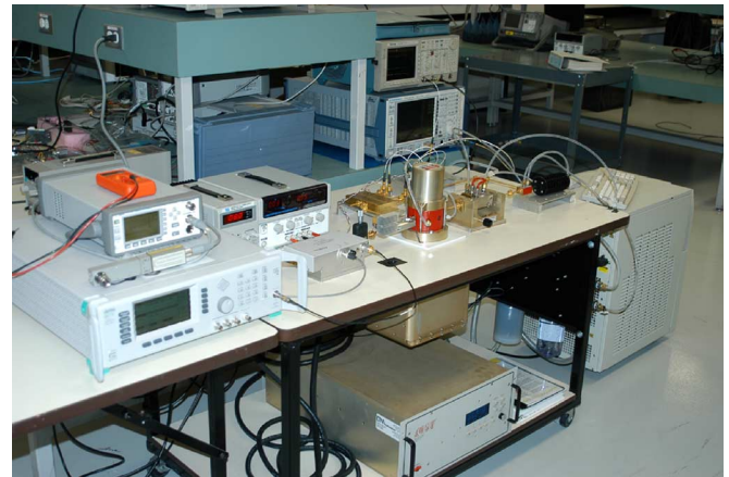
Fig. 14. Phase-noise measurement setup.
