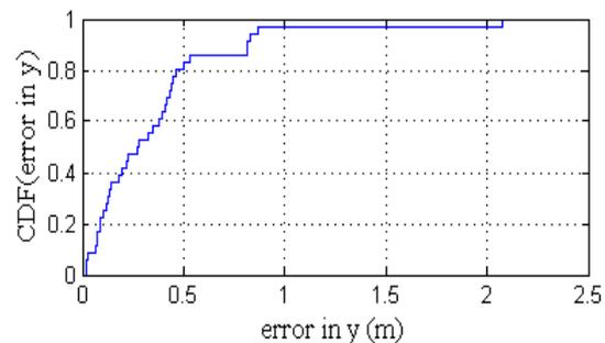
Fig.6: CDF for the error in 'y', MLP testing, LOS.
