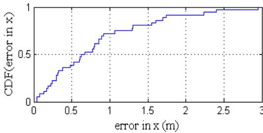
Fig. 8: CDF for the error in 'x', GRNN testing, LOS.
