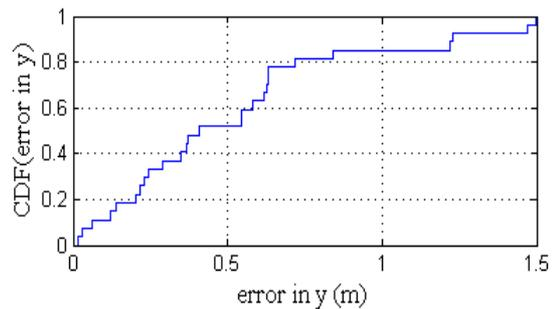
Fig.18: CDF for error in 'y', GRNN testing, NLOS
