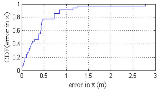
Fig.4: CDF for the error in 'x', MLP testing, LOS.
